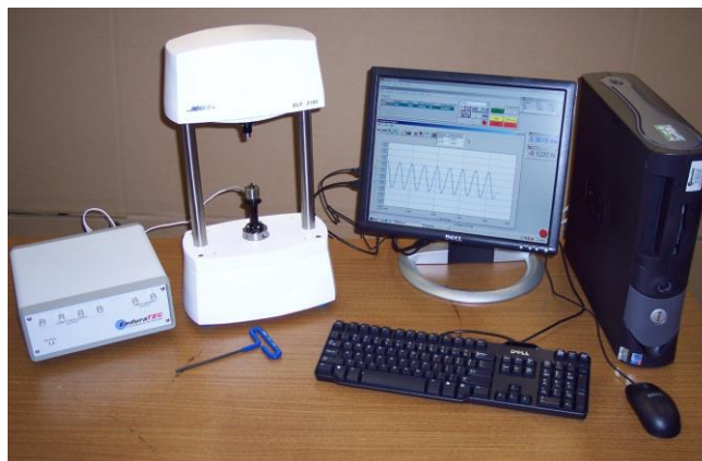
Figure 3. Bose ElectroForce dynamic tester up to 22N for stent testing, model 3100
